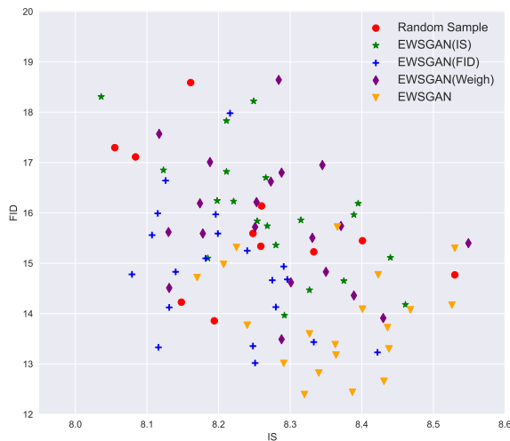
Fig. 9. Final populations in the objective space under various scenarios. The closer the points in the graph are to the bottom-right corner, the better the network. Some randomly sampled solutions are not depicted as they would fall outside the represented window.
